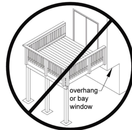
Figure 18: No Attachment to House Overhang
